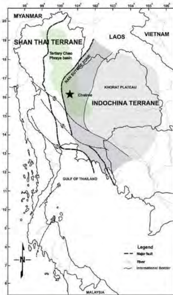
Figure 1 Map of Thailand, showing the location of the Chatree deposit in which Thailand's Loi-Phetchabun Volcanic belt is bound by the Nan and Loi Suture zones. The volcanic belt represents the remnant oceanic and continental arc complexes that developed prior and associated with the suturing of the Shan-Thai and Indochina Terranes (modified from Chausiri, 2000).
