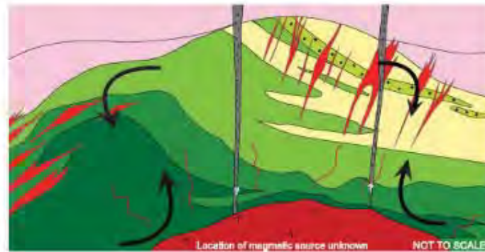
Scenario # 1: Magmatic source is younger than host and location of mineralization is controlled by host rock competency
